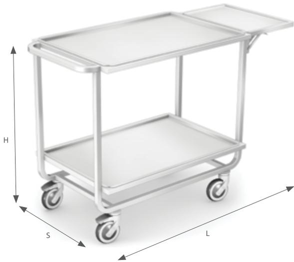
**WPP series trolleys** are made entirely of stainless steel grade 0H18N9 (AISI 304), equipped with castors with a diameter of 125 mm, including two with lock **top/shelf** in the form of one or two removable trays
