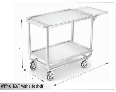
WPP series trolleys are made entirely of stainless steel grade 0H18N9 (AISI 304), equipped with castors with a diameter of 125 mm, including two with a blockade top / shelf in the form of one or two removable trays
