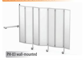
Elements of **PH series screens** are made of: **frame** of aluminium, powder coated in colour according to RAL palette, folding, equipped with castors with a diameter of 75 mm **filling** of a white plastic plate (PC polycarbonate)
