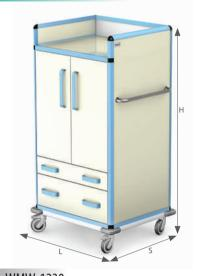
Elements of **WMW** series trolleys are made of: frame of closed aluminium profiles and ABS connectors, anodized or powder coated in the colour according to RAL palette TECH-MED sample-card filling of chipboard laminated on both sides top of chipboard, enclosed on three sides steel base, powder coated; equipped with castors of 100 mm diameter, including two with a blockade, base with buffers at the corners
